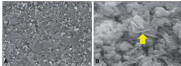
**Fig. 2.** OCP attached to the surface of the bovine bone. **A.** Scale-shaped OCPs were shown on the surface of the bone graft material ( $\times 5000$ , SEM). **B.** OCP was embedded among the round-shaped bone particles (yellow arrow  $\times 50000$ , SEM). Each gradation on the scale indicates 1  $\mu\text{m}$ .
